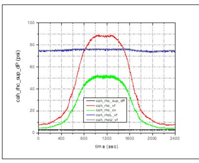
It has been suggested that if the modulating valve at the exit of the loop is wide open, that the exit flow will be equal to the sum of the flows to the coils. This is clearly not the case. Three separate balance valves are required to fully balance and characterize the system.
